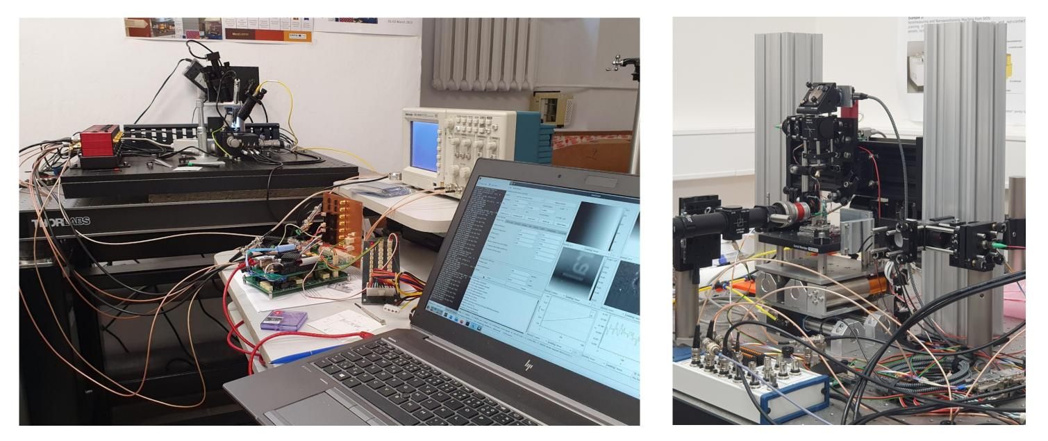
Picture on the left shows how Gwyscope is used to control a custom built SPM system such as Thorlabs EDU-AFM kit. Photo of CMI's custom built Image on the left shows topography of a BudgetSensors reference sample grating. MetExSPM sample detail is on the right. Feedback loop was affected by performance of particular AFM probe after a few hours of searching for the right location. Acquired with Gwyscope & Thorlabs EDU-AFM.
