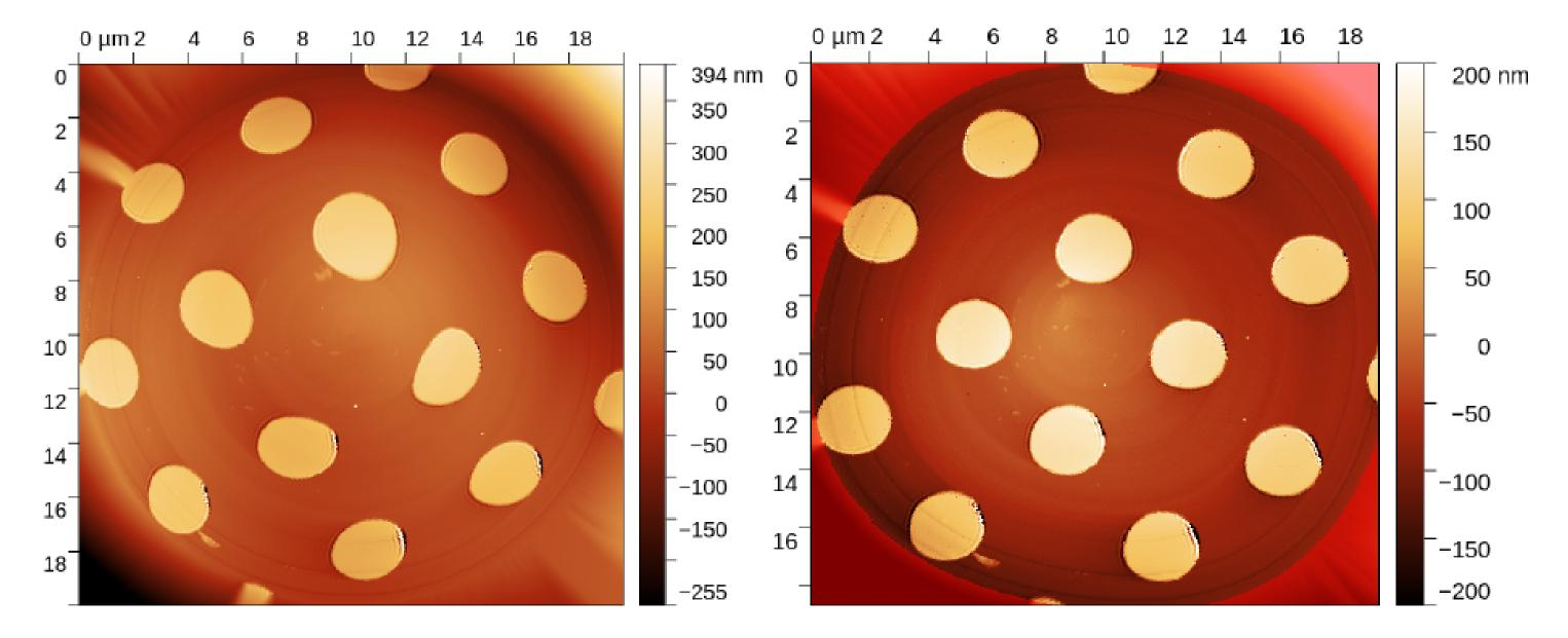
BudgetSensors reference sample dots grating. Comparison of piezo data use (left) and strain gauge data use (right) for spiral scan path. Acquired with Gwyscope & Thorlabs EDU-AFM.
