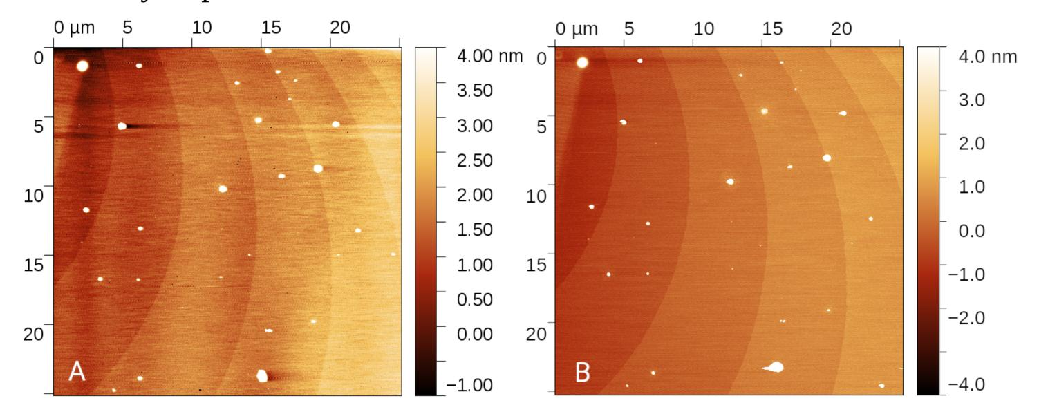
Comparison of measurements on silicon steps. Acquired using a custom built setup with Gwyscope (A). The same area was measured on Bruker Dimension Icon commercial AFM (B).
